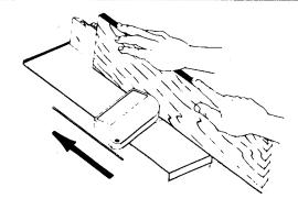
Always feed WITH THE GRAIN whenever possible. If the nature of the work piece is such that it must be fed AGAINST THE GRAIN, take very light cuts and feed slowly.
